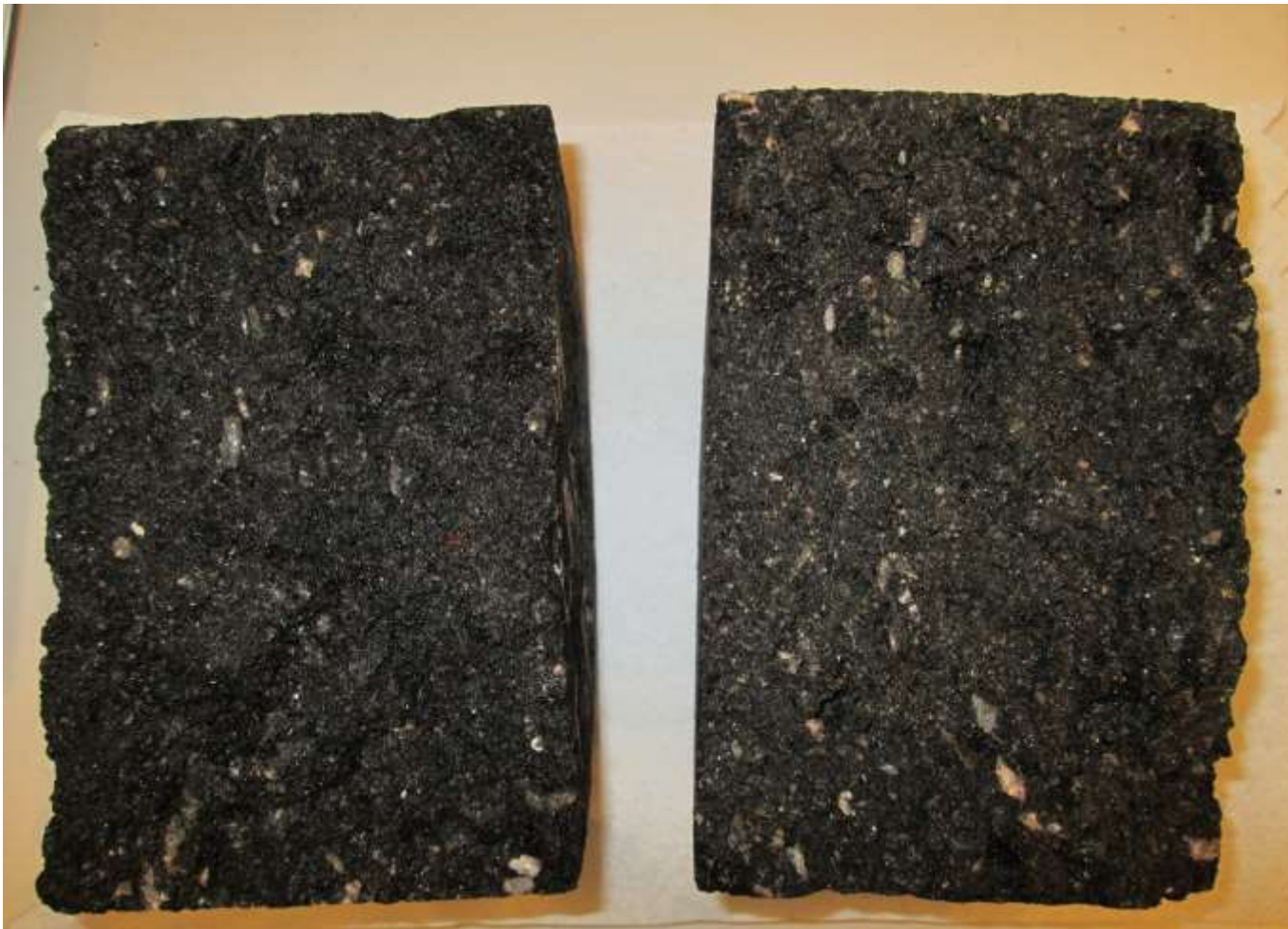
Fractured TSR Specimens with TSR of 60. The Conditioned sample is on the right and the dry on the left.
